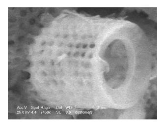
Figure: SEM image of a single frustule of as-received diatomaceous earth.
