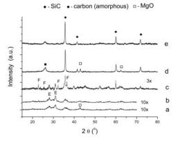
XRD patterns of Sepiolite B/novolac samples heat treated at:
