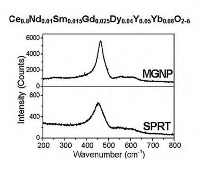
Figure: Raman spectra of nanopowders obtained by MGNP and SPRT methods.
