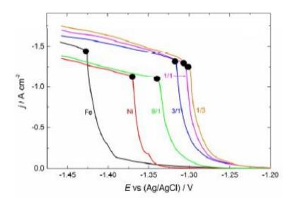
Figure: The polarization diagram for the Fe-Ni powders electrodeposition recorded at a sweep ratio of 1mV s<sup>-1</sup> (after IR drop compensation) for different Ni/Fe ions concentration ratios (marked in the figure).
