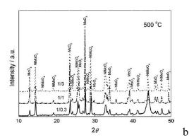
Figures: (a) The polarization diagrams for the Ni–Mo–O powders electrodeposition recorded at a sweep rate of 1mVs<sup>-1</sup> (after IR drop compensation) for different Ni/Mo ions concentration ratios; (b) The diffractograms for the powders annealed at 500 °C electrodeposited at different Ni/Mo ions ratios (marked in the figure); (c) The SEM micrograph of the asdeposited powders for the Ni/Mo=1/3.
