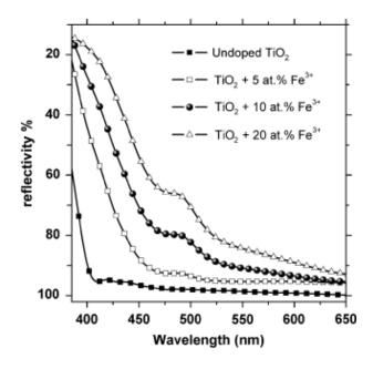
Figure: UV/Vis reflectance spectra of pure TiO<sub>2</sub> and TiO<sub>2</sub> doped with different at.% of Fe<sup>3+</sup> ions, indicated in the figure.
