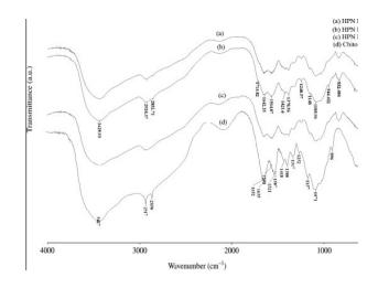
Figure: FTIR spectra of HPN I-1, HPN I-4, HPN II-5 and chitosan.
