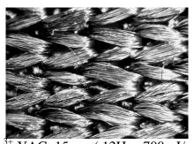
Figure: ACC, Er <sup>3+</sup>:YAG, 15 sec (.12Hz, ,700mJ/pulse); Magn.x28.
