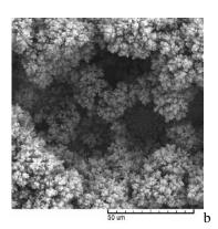
Figure: (a) Copper deposit obtained at an overpotential of 1,000 mV; (b) the coalesced hole and (c) non-coalesced obtained by PO regime electrolysis with a pause duration of 5 ms.
