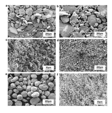
Figure: SEM. Morphology of Cu-2 wt.%Al<sub>2</sub>O<sub>3</sub>, Cu-4 wt.%Al<sub>2</sub>O<sub>3</sub> and Cu\*-4wt.%Al<sub>2</sub>O<sub>3</sub> composite powders. (a–c) After 3 h and (d–f) after 20 h of milling.
