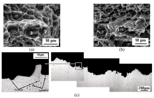
Figure: SEM micrographs showing fracture surfaces (a, b) and characteristic fragment of fracture surfaces of alloy 1 observed by OM (c). Phases: 1- Mg<sub>2</sub>Si, 2-(Cu,Fe,Mn)Al<sub>3</sub>, 3-Al<sub>7</sub>Cu<sub>2</sub>Fe.
