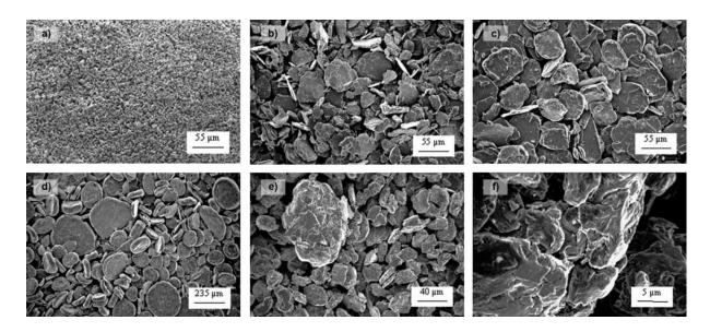
Figure:SEM.Morphology of as-received and milled Cu-3 wt.% Al particles: (a) as-received; (b) 3 h; (c) 5 h; (d) 10 h, (e) 20 h, (f) detail of figure (e).
