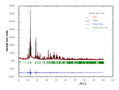
Figure: XRPD pattern after refinement procedure using Rietveld's method.
