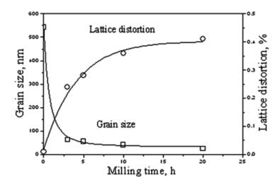
Figure: Effect of milling time on grain size and lattice distortion of Cu-3 wt.% Al.
