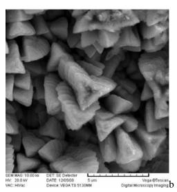
Figure: (a) Christmas tree-like crystals; (b) crystals of the shape of triangles.
