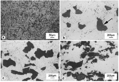
Figure: Microstructure of the tested materials: a) ZA-27 alloy, b) composite 3% Al<sub>2</sub>O<sub>3</sub>, c) composite 5% Al<sub>2</sub>O<sub>3</sub> and d) composite 10% Al<sub>2</sub>O<sub>3</sub>.
