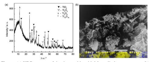
Figure: (a) XRD pattern of titanium oxide with Magneli phase structure. (b) SEM image of titanium oxide with Magneli phase structure.
