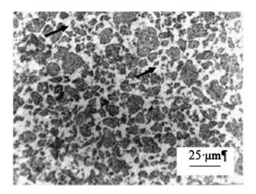
Figure: Light micrograph. Microstructure of Cu-4 wt.% Al<sub>2</sub>O<sub>3</sub> compact. Arrows indicate the recrystallization areas occurred during hot pressing.
