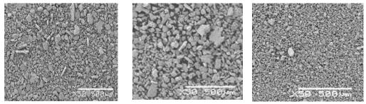
SEM micrograph. Morphology of Cu-4 wt.% TiB<sub>2</sub> particles after different milling time; (a) 5h, (b) 10h and (c) 20 h
