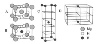
Figure: Unit cells of investigated compounds a) pureMgH<sub>2</sub>, b) MgBH<sub>4</sub>, c) Mg<sub>4</sub>BH<sub>10</sub> and d) Mg<sub>15</sub>BH<sub>32</sub>. For c) and d) only unit cells' stacking is shown, with positions of boron atoms.
