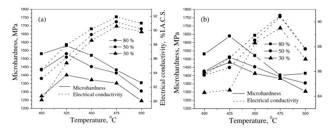
Figure: Effect of prior cold deformation and aging temperature on hardness and electrical conductivity; (a) Cu-Cr-Zr; (b) Cu-Cr-Zr-Mg. Aging time-2h.
