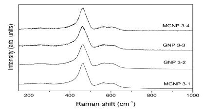
Figure: Raman spectra of nanopowders obtained by GNP and MGNP methods with different glycine/nitrate ratio.
