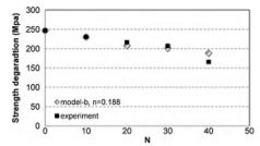
Figure: Strength degradation (model with damage inside the sample) versus number of cycles (*N*).
