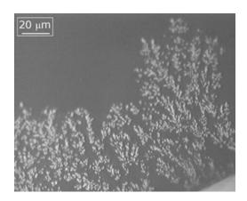
Figure: Cross-section of a copper deposit electrodeposited from  $0.15~M~CuSO_4$  in  $0.50~M~H_2SO_4$ , at an overpotential of 1000~mV with a quantity of the electricity of  $10~mA~h~cm^{-2}$ .
