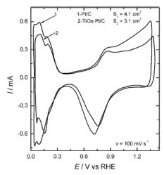
Figure: Cyclic voltammogram of Pt/C and TiOx–Pt/C electrodes (0.1 V s<sup>-1</sup>) in nitrogen-purged 0.5 mol dm<sup>-3</sup> HClO<sub>4</sub> solution at 25 °C.
