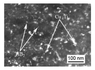
Figure: TEM. TiB<sub>2</sub> particles and Cu<sub>4</sub>Ti equilibrium precipitates in the copper matrix.
