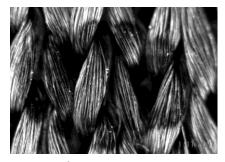
Figure: Effect of 15 pulses 60J/cm2 Nd<sup>3+</sup>: YAG laser, spot 2mm on carbon material P7295-2.
