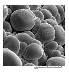
Figure: Typical powder particles for all as-deposited Fe–Ni powders. All powders were deposited at the current density of 2.5 A cm<sup>-2</sup>.
