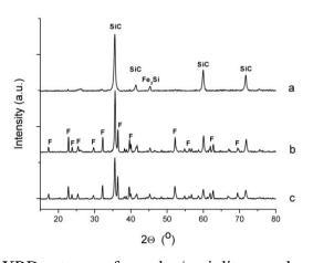
XRD patterns of novolac/sepiolite samples heat treated at 1673K: a) C/SiO<sub>2</sub>=8, b) C/SiO<sub>2</sub>=4, c) C/SiO<sub>2</sub>=2; (F-forsterite)
