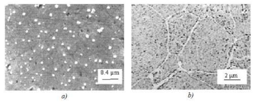
Figure: SEM and light microscopy. (a) SEM micrograph of polished Cu-2 wt.% Al and (b) light micrograph of polished Cu-4 wt.% Al<sub>2</sub>O<sub>3</sub> compacts processed from 5 h milled powders.
