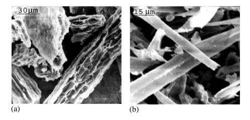
Figure: SEM micrograph of carbonized achenes chemically treated with NaOH (a) and pyrogallol (b).
