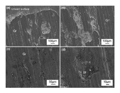
Figure: Wear surfaces of the composite in conditions of dry sliding for 50 N of applied load and 0.10 m/s of sliding speed.
