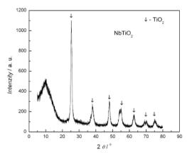
Figure: X-ray diffraction spectra of Nb–TiO2 substrate with specified composition.
