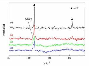
Figure: The diffractograms for the powders electrodeposited at different Ni/Fe ions ratios (marked in the figure).
