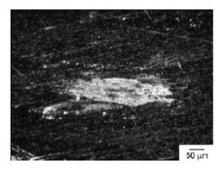
Figure: Wear track on Ti-6Al-4V alloy sample at 1000x magnification.
