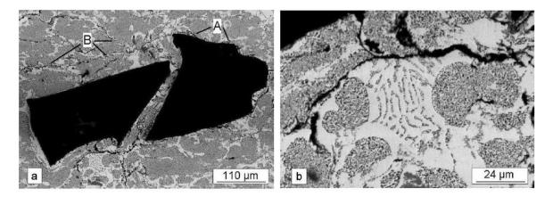
Figure: Microstructure of Zn25Al3Cu/Al<sub>2</sub>O<sub>3</sub> composite (3 wt. % Al<sub>2</sub>O<sub>3</sub>), SEM, polished. (a) interface and microcracks; (b) microcracks development.
