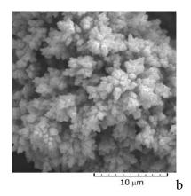
Figures: (a) The honeycomb-like copper structure; (b) agglomerate of copper grains obtained with a deposition pulse of 20 ms. Deposition time: 185 s; (c) Cross-section of the copper deposits obtained with deposition pulse of 20 ms.
