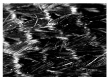
Figure: Light microscope ACC, alexandrite laser, 5 pulses, spot 10mm, 36J/cm<sup>2</sup> Magn.x84.
