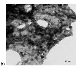
Slika: TEM snimci sintetisanih nanoprahova dobijenih SPRT metodom: (a)  $Ce_{0.8}Nd_{0.01}Sm_{0.04}Gd_{0.04}Dy_{0.04}Y_{0.07}O_{2-\delta}$ , (b)  $Ce_{0.8}Sm_{0.005}Gd_{0.005}Dy_{0.095}Y_{0.095}V_{0.095}O_{2-\delta}$ .
