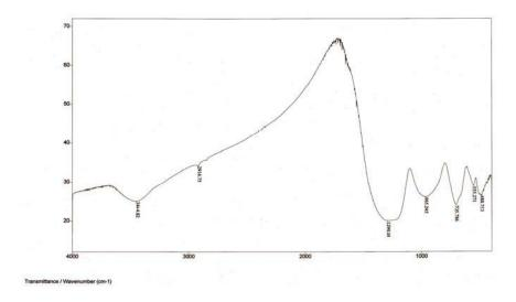
Figure: IR spectrum of glass ceramics.
