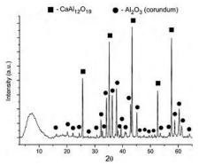
Figure: XRD pattern of the castable matrix sample sintered at 1600 °C/3 h.
