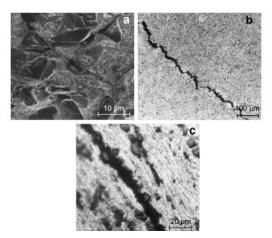
Figure: Fracture surface of DRA alloys after 60 min of homogenization. (a) SEM: CW67–10 vol.% SiC,  $d_{SiC} = 10 \mu m$ ; (b) OM: CW67–10 vol.% SiC,  $d_{SiC} = 10 \mu m$ ; (c) OM: CW67–10 vol.% SiC,  $d_{SiC} = 10 \mu m$ .
