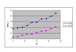
Figure:Damaged surface level (P/P<sub>o</sub>) versus number quench experiments (N).
