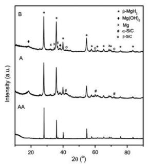
Figure: XRD patterns of commercial MgH<sub>2</sub> powder (AA) and MgH<sub>2</sub> milled with 5 wt % of different SiC phases: α-SiC (A) and β-SiC (B).
