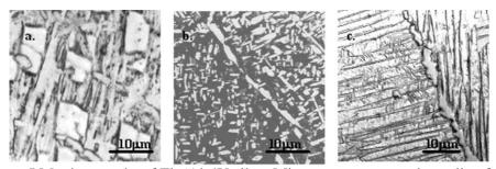
Figure: LM micrographs of Ti-6Al-4V alloy. Microstructure upon air-cooling from: (a) 1100 °C; (b) 1050 °C; (c) 950 °C.
