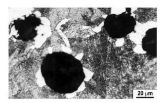
Figure: LM. Microstructure of as-cast ADI specimen.
