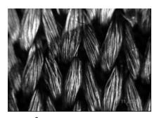
Figure: Effect of 5 impulses 36 J/cm<sup>2</sup> Alexandrite laser, spot 10mm on carbon fiber material.
