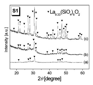
Figure: XRD patterns of directly synthesized La<sub>9.33</sub>(SiO<sub>4</sub>)<sub>6</sub>O<sub>2</sub> during combustion process.
