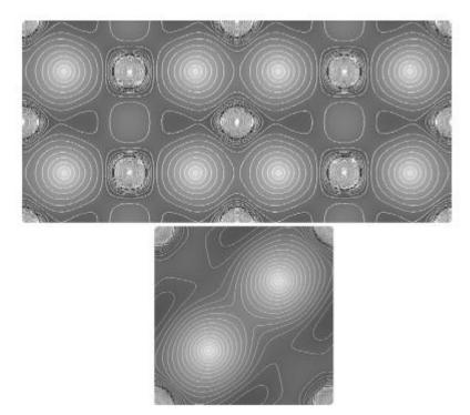
Figure: Valence electron charge densities in [110] (upper) and [100] (lower) crystal planes of the MgH<sub>2</sub> unit cell.
