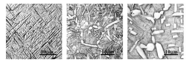
Figure: Light microscope. Microstructure of Ti-6Al-4V alloy upon water-quenching from: (a) 1100 °C; (b) 950 °C; (c) 900 °C
