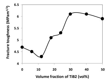
Figure: Effect of TiB<sub>2</sub> volume fraction on fracture toughness of SiC-TiB<sub>2</sub> composite sintered at 1940 °C for 1h.
