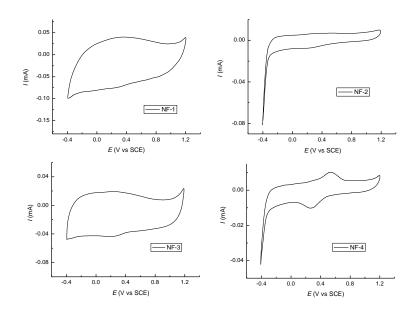
Figure: Cyclic voltammograms of natural fibers applied on glassy carbon electrode in 0.1 M HClO<sub>4</sub> solution; sweep rate 100 mV/s.
