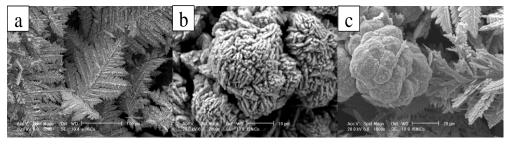
Figure: Morphology of Ni-Co powders electrodeposited from electrolytes containing: (a)  $Ni^{2+}/Co^{2+} = 1.00$ ; (b)  $Ni^{2+}/Co^{2+} = 0.50$ ; (c)  $Ni^{2+}/Co^{2+} = 0.33$ .
