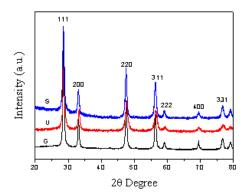
Figure: XRD patterns of CeO<sub>2</sub> powder sample obtained by combustion synthesis.
