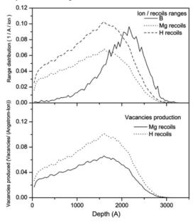
Figure: Results of Monte Carlo simulations of 45 keV B ions irradiation of MgH<sub>2</sub> obtained by SRIM 2003 package. (Top): depth distribution of incident ions and recoiled atoms, (Bottom): vacancies production as a function of depth.
