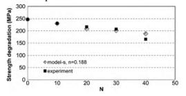
Figure: Strength degradation (model with surface damage) versus number of cycles (*N*).
