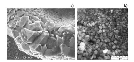
Figure: The view of a crater rim (a) and periphery (b) of irradiated surface on the super-alloy Inconel 600 (160 fs laser pulse, laser energy 19 nJ, irradiation time 7 min, pulse repetition rate 75 MHz, SEM analysis).
