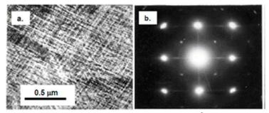
Figure: TEM micrograph of Cu-2Be after aging at 250 °C for 120 h. (a) "Tweedlike" microstructure; (b) SADP showing continuous streaks in (001) direction. Thin foil.
