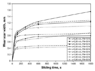
Figure: Wear curves of ZA27 HT5 alloy at different specific loads and sliding speeds.
