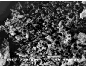
SEM micrographs of SiC obtained from novolac/sepiolite mixture (C/SiO<sub>2</sub>=8)
