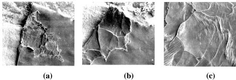
Figure: Amorphous material,70%Ti-30%Fe: (a)-Damage view, SEM 50x (b); detail from (a), SEM 500x; (c) detail from (a), 198x.
