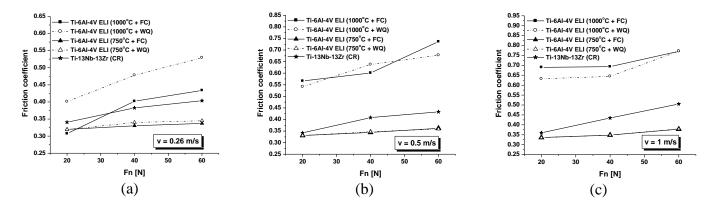
Figure: Friction coefficient of cold rolled Ti-13Nb-13Zr and heat treated Ti-6Al-4V ELI alloys as a function of applied load at the sliding speed of 0.26 (a), 0.5 (b) and 1.0 m/s (c).
