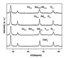
Figure: XRD patterns of nanometric doped ceria powders.
