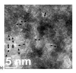
Figure: TEM images of synthetisized nanopowders obtained by MGNP method: (a)  $Ce_{0.8}Nd_{0.01}Sm_{0.04}Gd_{0.04}Dy_{0.04}Y_{0.07}O_{2-\delta}$ , (b)  $Ce_{0.8}Sm_{0.005}Gd_{0.005}Dy_{0.095}Y_{0.095}O_{2-\delta}$ .
