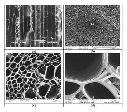
Figure: SEM microphotographs of porous silica ceramics obtained at 1300\_C for 4 h: (a) cross-section parallel to axial direction, (b–d) cross-sections perpendicular to axial direction.
