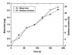
Figure: Mass loss and surface erosion during the cavitation testing.
