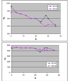
Figures: Values of longitudinal (Vp) and transversal (Vs) ultrasonic velocity during testing.
