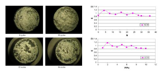
Figure: Samples KZ30 under thermal shock experiments, white area is non-damaged surface.
