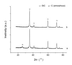
XRD patterns of SiC powders obtained from asbestos after 1873 K treatment: (a) washed with HF, (b) washed with HF and oxidized at 873K
