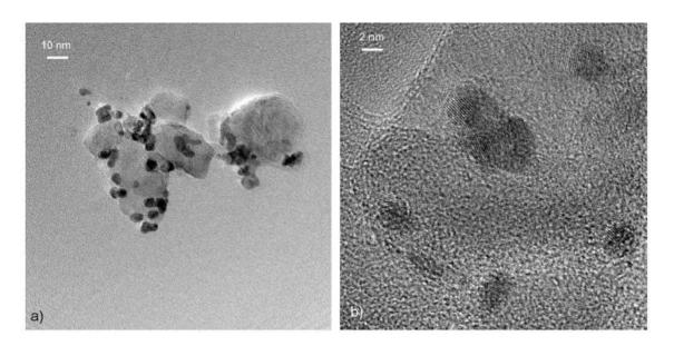
Figure: (a) TEM image of Pt–Ru nanoparticles on Nb–TiO2 support at low resolution, (b) HRTEM image of the same sample.
