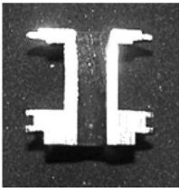
Figure: Photographs of the erosion paths at cut anodes: (a) Metco7 MB, 25–35 kW (courtesy of Inst. Nuclear Science, Vinca) and (b) PJ-100, 80–100 kW.
