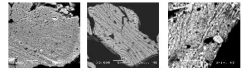
SEM micrograph. Microstructure of Cu-4 wt.%  $TiB_2$  powder particles after different milling time; (a) 5h, (b) 10h and (c) 20 h
