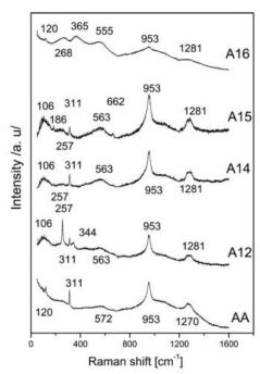
Figure: Raman shift of a commercial (AA)  $MgH_2$  powder, and samples irradiated using 120 keV  $A^{r8+}$  ions, with ion fluencies of  $10^{16}ions/cm^2(A16)$ ,  $10^{15}ions/cm^2$  (A15),  $10^{14}ions/cm^2$  (A14)  $10^{12}ions/cm^2$  (A12).
