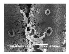
Figure: SEM micrograph of woodlike SiC ceramics.
