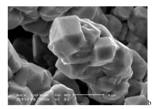
Figure: (a) Particle size distribution of copper powder particles obtained by reversing currents (sieve analysis); (b) SEM photomicrograph of copper powder particles obtained by reversing currents. Cathodic-to-anodic time ratio 2.5. Cathodic pulse duration 1s. Anodic pulse duration 0.4s. Cathodic (anodic) amplitude current density and average current density  $j_c=j_a=36 \text{ A/dm}^2$ ,  $j_{av}=15.42 \text{ A/dm}^2$ .
