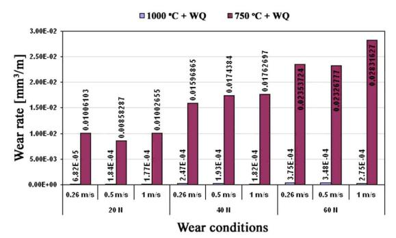
Figure: Effect of heat treatment on Ti-6Al-4V ELI alloy wear rate.
