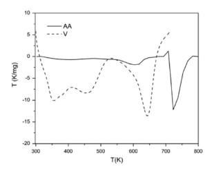
Figure: DTA curves of a commercial MgH<sub>2</sub> powder (AA) and MgH<sub>2</sub>–VO<sub>2</sub>(B) composite (V). Catalyzed system shows three maxima positioned at 642 K (HT), 456 K (IT) and 354 K (LT).
