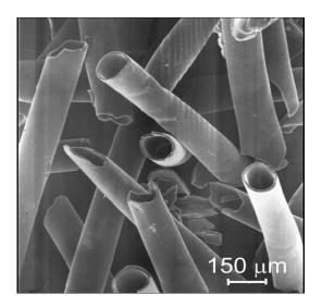
Figure: SEM micrograph of activated carbon hollow fibers obtained from polysulfone precursor.
