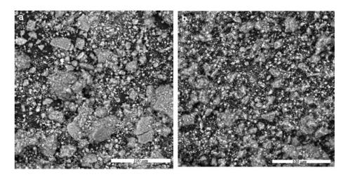
Figure: (a) SEM BSE micrographs of MgH<sub>2</sub>/a-SiC composites. (b) SEM BSE micrographs of MgH<sub>2</sub>/b-SiC composites.
