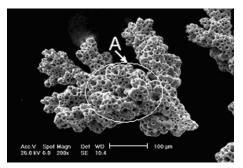
Figure: SEM photographs of morphology of cobalt powder particles deposeted onto (a) glassy carbon; (b) cobalt and (c) nickel electrode.
