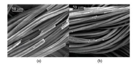
Figure: SEM Microphotographs of ACC $\gamma$  from: a) side directly exposed to the  $\gamma$ -radiation; b) the opposite side.
