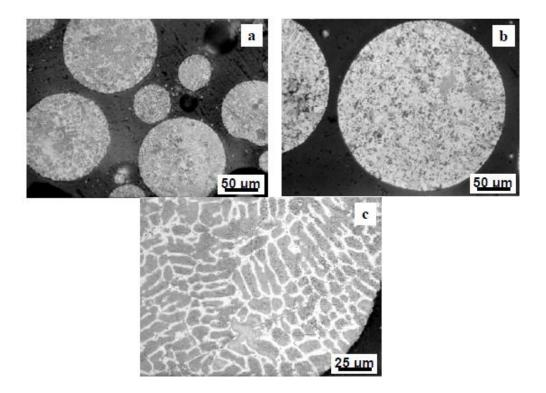
Figure: LOM micrographs showing the microstructure of different as-atomized Cu-0.6Ti-0.02B-2.5TiB $_2$  (wt.%) alloy powder sieved to fractions: (a) d < 80  $\mu$ m, (b) 80  $\mu$ m< d < 150  $\mu$ m and (c) 200  $\mu$ m< d < 315  $\mu$ m.
