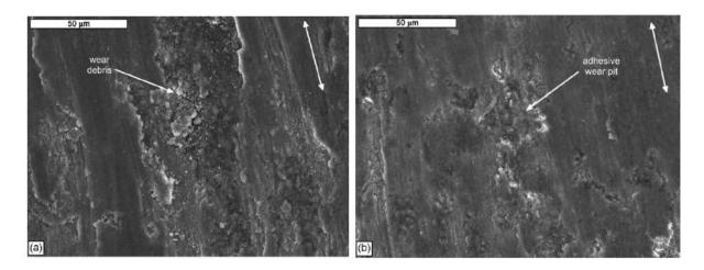
Figure: SEM micrographs of test samples worn surfaces (a) A356 aluminium alloy and (b) composite C1 (with 10 wt.% Al<sub>2</sub>O<sub>3</sub> particles); sliding directions is denoted with double arrows.
