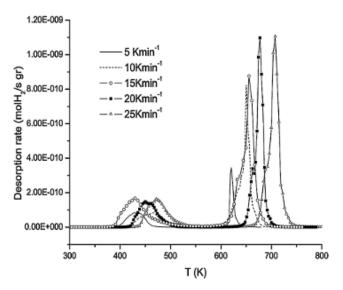
Figure: H-desorption rate curves for  $MgH_2$ – $CeO_2$  at different heating rates. 5 K/min (solid line) 10 K/min (dash line), 15 K/min (empty circle), 20 K/min (filled square), 25 K/min (empty triangle).
