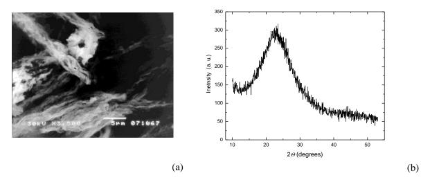
Figure: Scanning electron microscopy (SEM) image (a), and X-ray diffraction (XRD) pattern (b) of silica material SBA-15.
