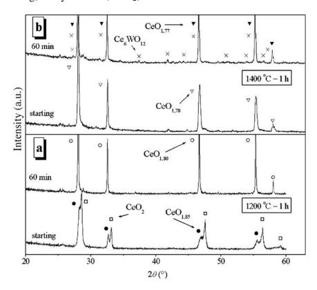
Figure: Phases identified in starting and milled  $CeO_2$  powders fired for 1 h at (a) 1200 °C and (b) 1400 °C.
