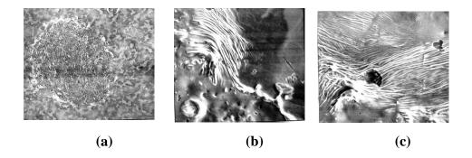
Figure: Tin plate: (a) Damage view, 28x; (b) bottom of the damage and nondamaged material, 500x (c); wall and the bottom of the crater, 660x.
