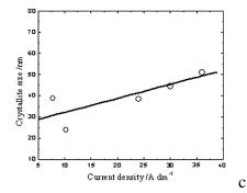
Figure: SEM microphotographs (a) and (b) of copper powder particles deposited at current density  $j = 7.71 \text{ Adm}^{-2}$ ; (c) The dependence of crystallite size on current density.
