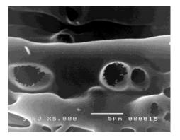
Figure: SEM mocrograph of biomorpic SiO<sub>2</sub> ceramics.
