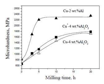
Figure: Effect of milling time on microhardness of hot-pressed composites:  $\triangle$  - based on internally oxidized Cu-2 wt.% Al prealloyed powder;  $\blacksquare$  - based on 30  $\mu$ m copper powder;  $\Delta$  - based on 15  $\mu$ m copper powder.
