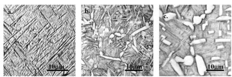
Figure: LM micrographs of Ti-6Al-4V alloy microstructure upon water-quenching from: (a) 1100 °C; (b) 950 °C; (c) 900 °C.
