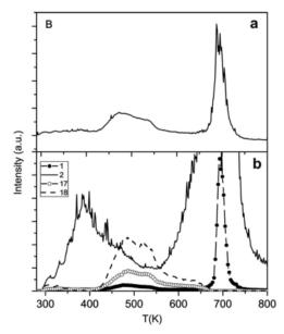
Figure: Results of TPD measurements, obtained at constant heating rate of 5 K/min, in the temperature range from RT to 973 K, of MgH<sub>2</sub>/ $\beta$ -SiC powder (B): a) total signal of all desorption products, b) separate signals of desorption products: 1(H+), 2 (H<sub>2</sub>),17(OH<sup>-</sup>) and 18 (H<sub>2</sub>O).
