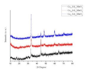
Figure: XRD patterns of  $Ca_{(1-x)}Gd_xMnO_3$  (x = 0,1; 0,2; 0,3) powder sample synthesized by sucrose-nitrate procedure (SNP).
