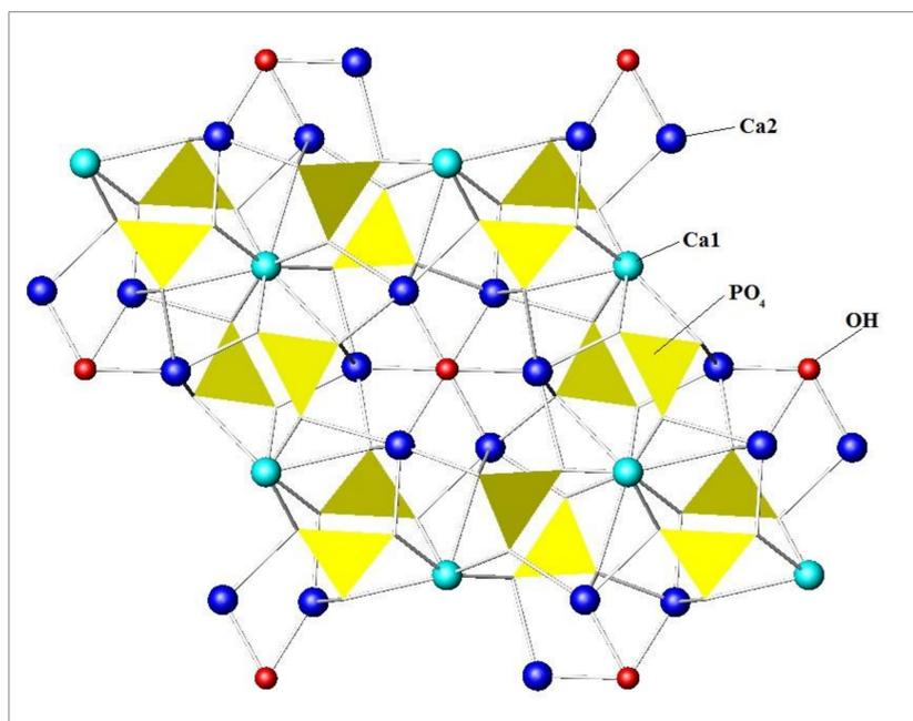
Fig. 1. Structure of Hydroxylapatite (HAp), s.g.  $P6_3/m$
