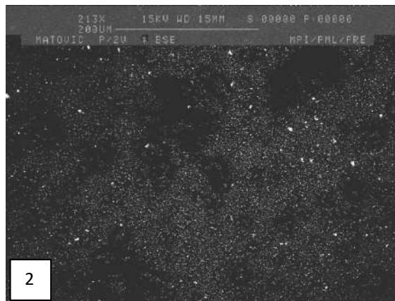
Figure 19. (a): Backscattered electron images of green compacts of yttrium - ( \text{LiYO}_2 containing \text{Si}_3\text{N}_4 mixtures prepared by planetary and attrition milling for 1h).
