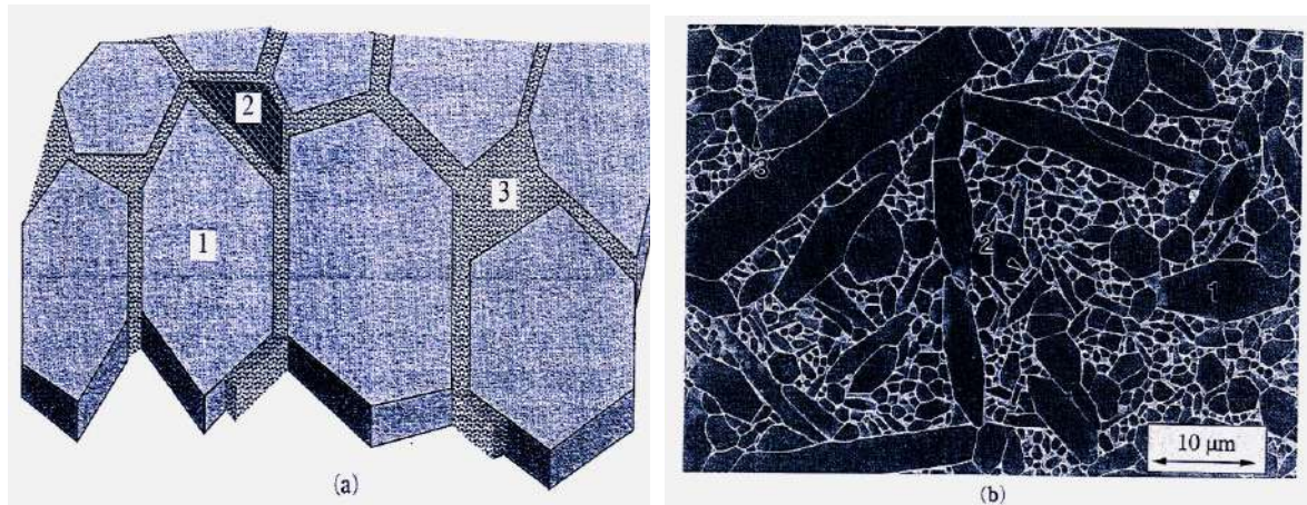
Figure 51. Typical microstructure of a liquid-phase sintered \text{Si}_3\text{N}_4 ceramics (schematic (a) and SEM micrograph (b)).
